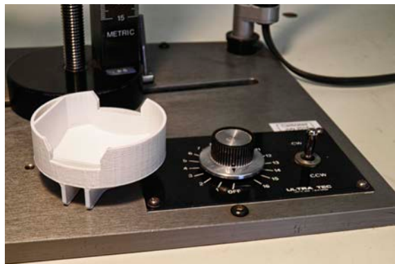
The Protractor Protective Cover, manufactured by Rich Yarborough, from the design by Dave Rose.
