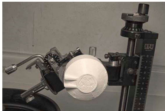
Ultra Tec Faceting machine with the Protractor Protective cover installed.
