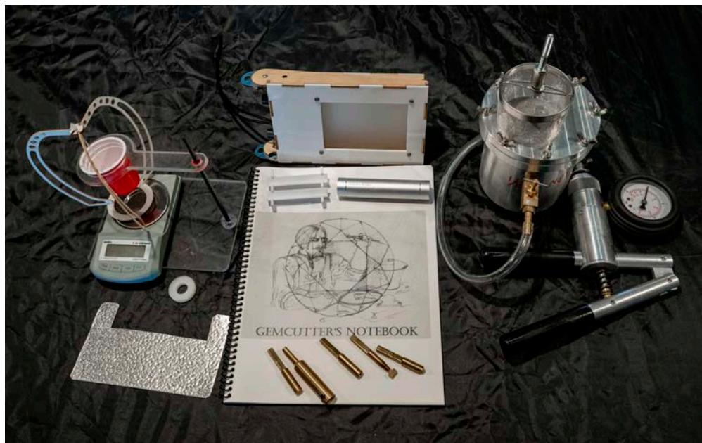
**Tools of the trade. Left to right:** Specific gravity machine; lap spacer; splash pan guard; gem cutter's light box and accessories; gem cutter's notebook; custom specialty dops, and non-keyed adapter; custom clarity enhancer vessel, and vacuum/pressure pump.
