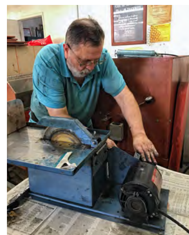
Fig. 7 Paul fixing the trim saw belt and pulley. Again, a greasy job!
